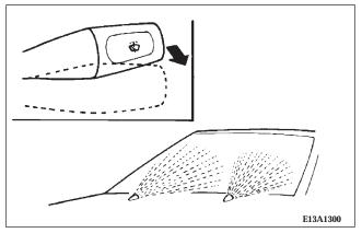
The windshield washer can be operated by pulling the lever toward you to spray fluid when the ignition key is in either the "ON" or "ACC" position.
